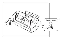
2 Remove the used ink film cartridge and holders.
